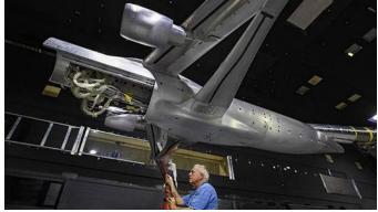
Researchers completed TTBW high-lift tests, including stability and control checks and groundeffects evaluations, in September at NASA Langley Research Center's 14 X 22-ft. subsonic wind tunnel in Hampton, Virginia. Credit: NASA
